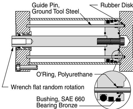
Two guide pins incorporated inside the cylinder pass through the piston head. These guide pins prevent rotation of the rod with a tolerance of  $\pm 1^\circ$ . The guide pins, being incorporated inside, are protected from the environment, physical damage, and are lubricated by the system lubrication, and require NO additional space, leaving the rod end area free for attachments and tooling as required by your application.
