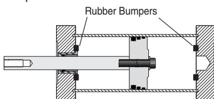
Standard rubber mass will compress and give full stroke at 60 to 80 psi. This mass can be adjusted to meet your specific pressure and/or dynamic load requirements.
