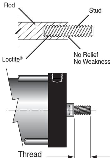
A high strength stud is threaded into the standard female rod end and retained with Loctite®. This method eliminates the small diameter thread relief area normally required when machining male threads. This provides a much stronger rod end which can be repaired, rather than replacing the complete rod, should the thread be damaged.
