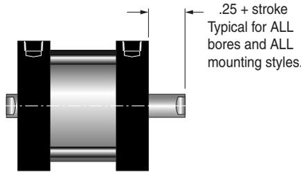
Standard piston rod and rod bushing on both ends of the cylinder.
