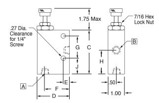
Super-Vee<sup>™</sup> Flow Control controls one direction – Free flow return
