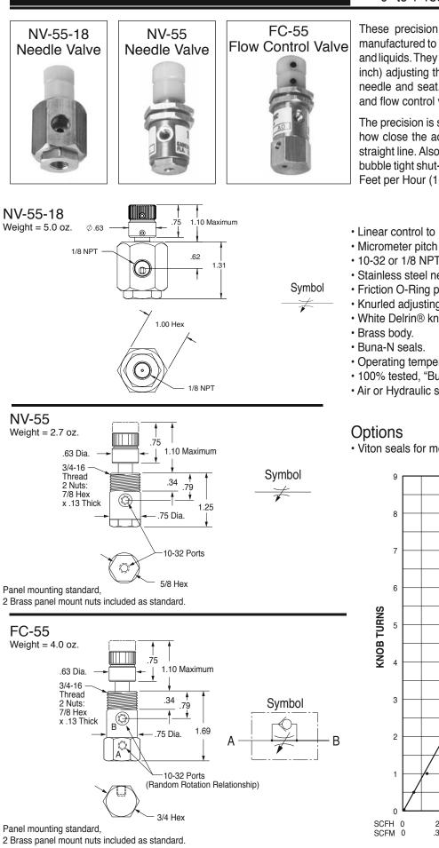
These precision machined valves are designed and manufactured to provide Micro-Fine™ control of gasses and liquids. They have a micrometer pitch (40 threads per inch) adjusting thread and precision machined tapered needle and seat. They are available as needle valves and flow control valves.
